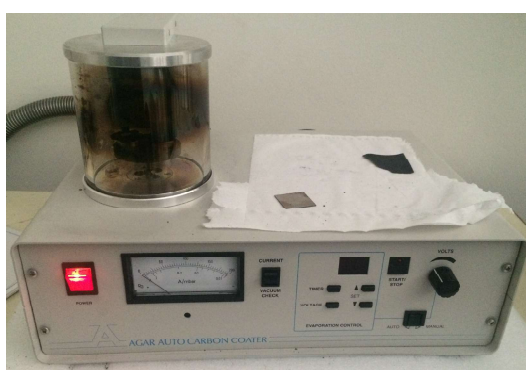
(b) Agar Automatic Carbon Coater
