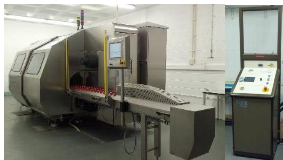
Figure 2. 29 – Images of two of hydrostatic high pressure equipments owned by the University of Aveiro. On the left is the Hyperbaric 55 with a 55 L capacity and on the right is the High-pressure U33 with a capacity of 100mL.
