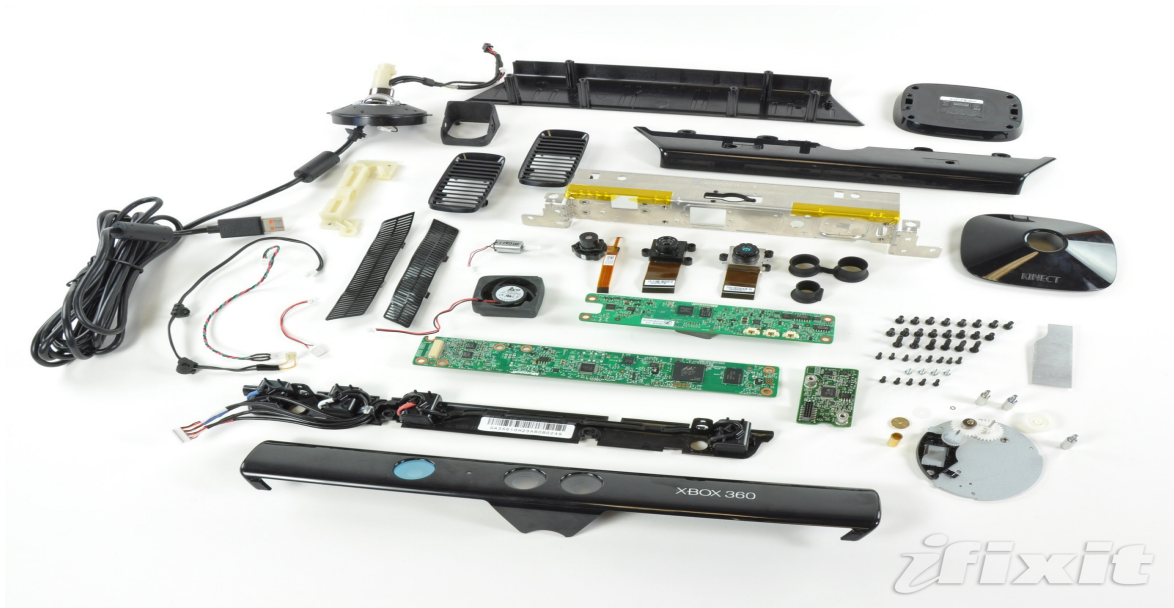
Figure 3.4: A disassembled Microsoft XBOX Kinect sensor [24].
