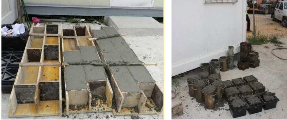
Figure 3.4 – Specimens preparation during the concreting on site
