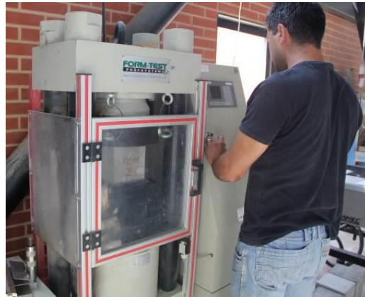
Figure 3.5 – Uniaxial compression tests
