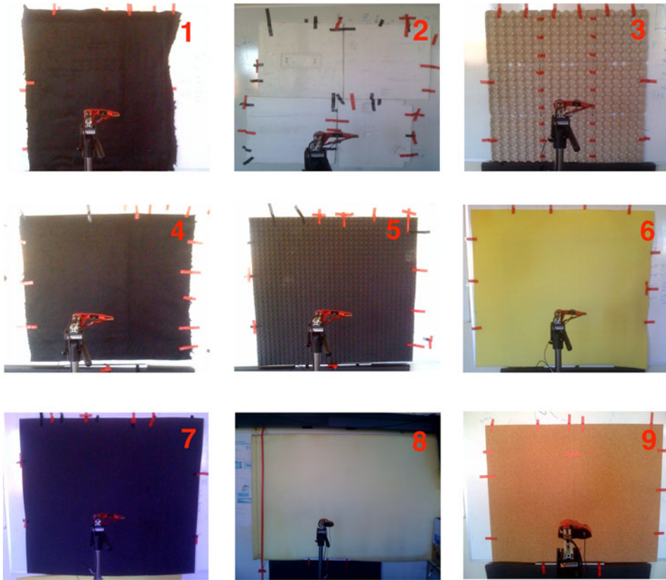
Figure 3. Materials used in the experiment 1, Felt fabric; 2, expanded polystyrene; 3, egg boxes; 4, coated egg boxes; 5, foamtek – pyramidal foam; 6, polyurethane foam 1 cm; 7, polyurethane foam 3 cm; 8, polyurethane foam 5 cm, 9, agglomerated cork sheet 5 mm.
