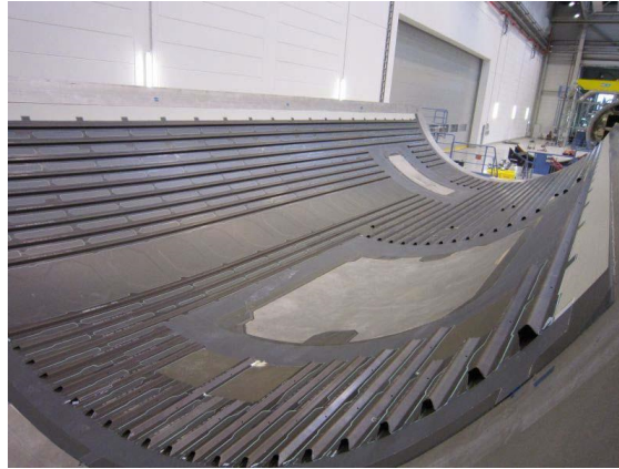
Figure 1.3: Composite stiffened panel applied in aerospace industry [21].
