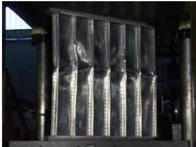
Figure 1.4: Failure of aluminium stiffened panel [7].
