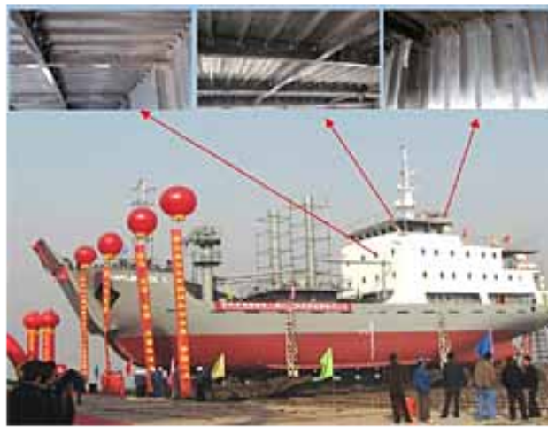
Figure 1.2: Aluminium stiffened panels applied in marine industry [16].
