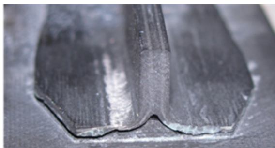
Figure 1.7: Adhesive failure of a composite stiffened panel [38].
