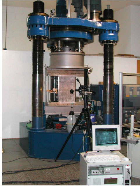
Figure 5.1: Buckling test facility [55].
