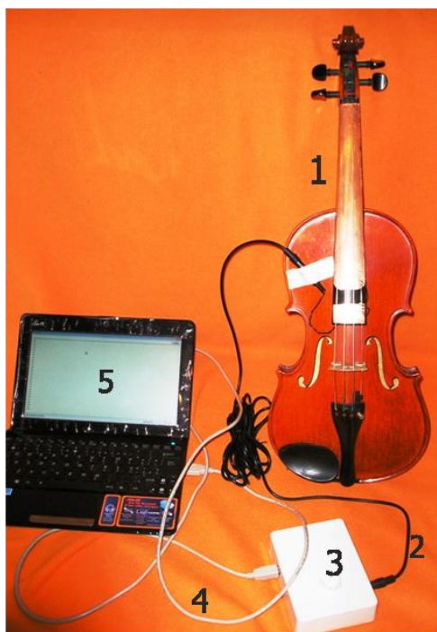
Figure 58. The basic structure of the sensor Filizzola/ Tramma
