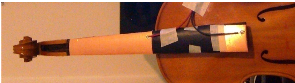
Figure 54. The “sandwich” composed of two copper tapes and one of Velostat in the middle on the violin fingerboard.
