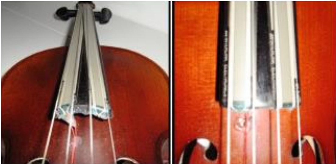
Figure 61. Sensor Force Sensing Resistor™ by 3M fixed on the fingerboard.
