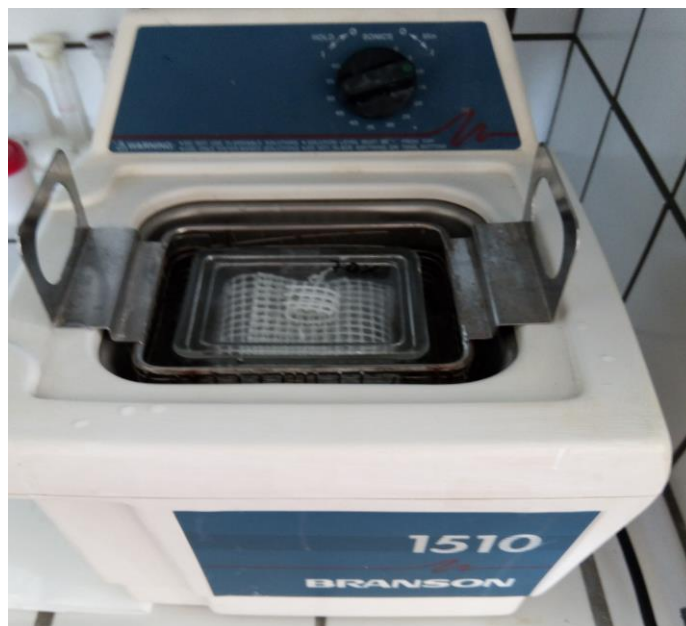
Figure 13. Preparing coverslips. Basket with coverslips, inside a glass staining jar, placed in the immersible ultra sonicator Branson 1510.
