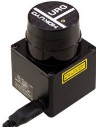
Figure 3.2: Laser Range Finder URG-04LX-UG01 used in the work.
