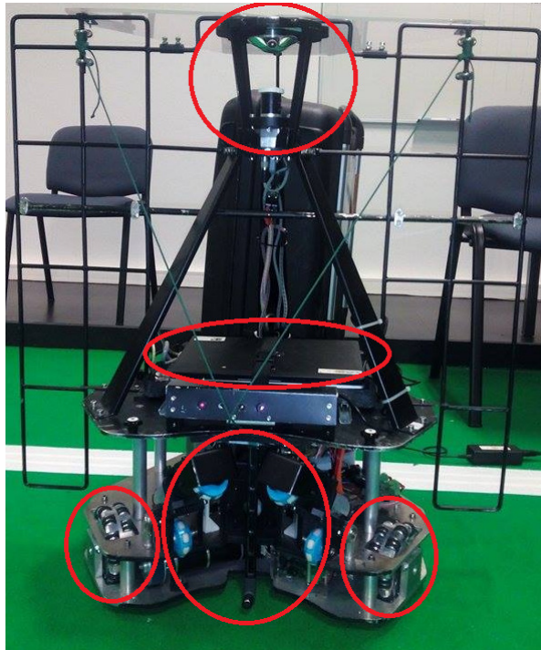
Figure 3.1: Current robot used in CAMBADA team. At the top it's the vision system, at the center the main processor unit. At the bottom, on the center it's the grabbers and kicker, and at the sides, are the wheels belonging to the locomotion hardware.
