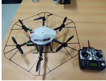
(b) AscTec Firefly hexadrone, a remote-controlled mobile robot.
