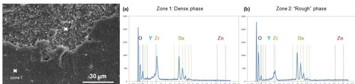
Fig. 4.29 - (a) SEM surface micrograph of reduced 0.96\text{BaZr}_{0.852}\text{Y}_{0.148}\text{O}_{3-\delta}+0.04\text{ZnO} ( 900^\circ\text{C} , 5 hours, flowing 10\%\text{H}_2 : 90\%\text{N}_2 ) and the correspondent energy spectra of the (b) dense and the (c) “rough” zones – mechanism b).
