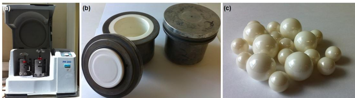
Fig. 3.3 – (a) High energy planetary ball mill (Retsch PM200), (b) 125 cm 3 tetragonal zirconia vials (Retsch) and (c) tetragonal zirconia balls with 10 mm and 15 mm of diameter (TOSOH Co.).
