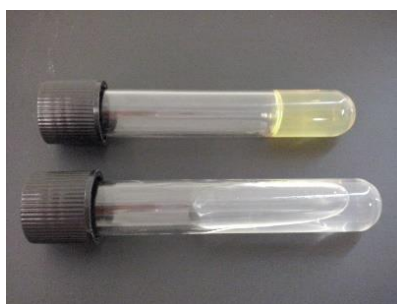
Figure 11. The effect of storage time on sample color. 12 % (w/V) WPI gels containing 0.9 \text{ mol L}^{-1} acetic acid, at pH 3.20 after being stored for one month (top) and one week (bottom).
