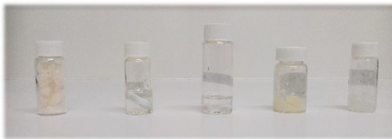
Figure 2.3. Macroscopic appearance of the synthesized Good's Buffer ionic liquids at 25°C. From the left to the right: [P 4444 ][MES], [P 4444 ][TES], [P 4444 ][CHES], [P 4444 ][HEPES], [P 4444 ][Tricine].
