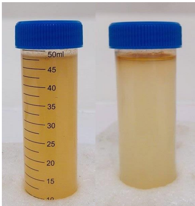
Figure 4.1. ABS composed of [P_{4444}][CHES] + salt + human urine (150 ng/mL of PSA added). ABS after being vigorously stirred (on the left) and after being centrifuged for 10 min and left in equilibrium for 15 min (on the right).
