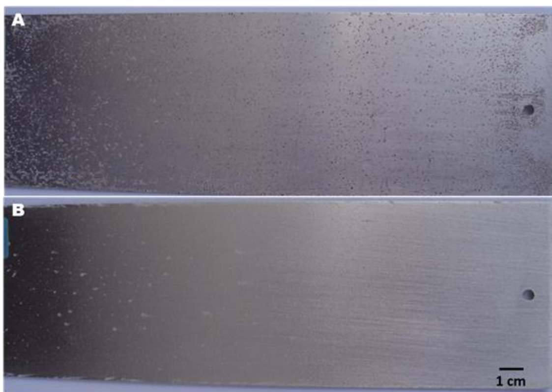
Figure 36: Coated AA2024 with (A) unmodified sol-gel and (B) with sol-gel containing MBT@PU-MC, after 168 hours in NSS.
