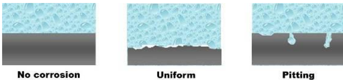
Figure 2: Differences between uniform and localized (pitting) corrosion.
