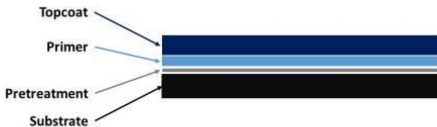
Figure 4: Schematic of components that make up an aircraft coating system, adapted from [24].
