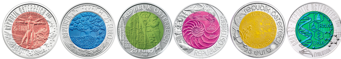
Figure 1.3 - Austrian Mint Silver Niobium coins, with coloured cores obtained by anodization of niobium [13].
