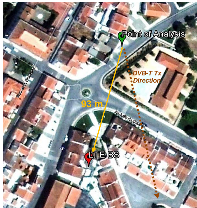
Fig. 4.19. Relative positions of the DVB-T receiver (point of analysis) and the LTE BS.
