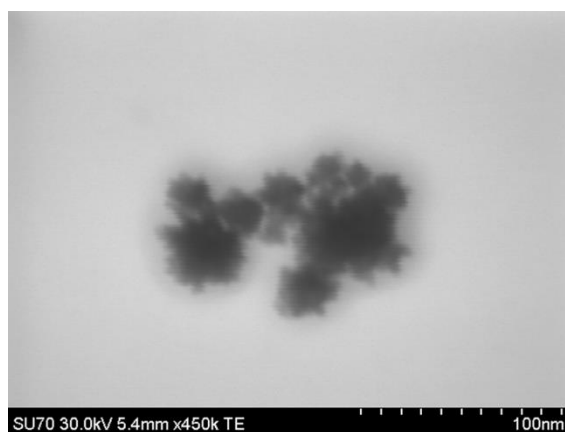
Figure 4.3 – SEM image of the star shaped nanoparticles in the gold colloid obtained by reduction with hydroxylamine.
