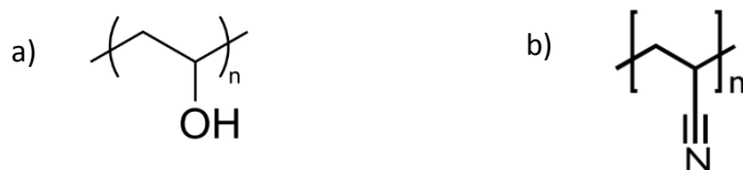
Figure 5.1 – Chemical structure of polymers used to produce electrospun fibres: a) poly(vinyl alcohol) and b) polyacrylonitrile.
