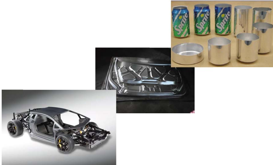
Figure 3.1: some examples of deep drawn pieces produced from aluminium alloy sheets
