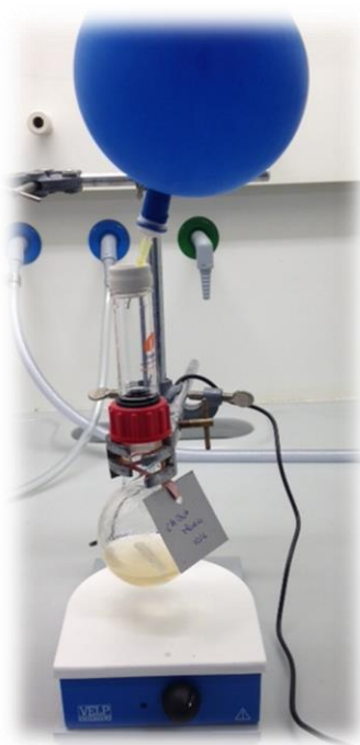
Figure 3.1. Synthesis of ionic liquids in an inert atmosphere.
