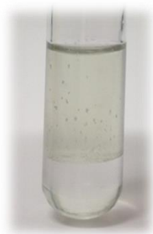
Figure 2.7. Visual appearance of the BSA extraction with an ABS formed by IL+ salt + water.
