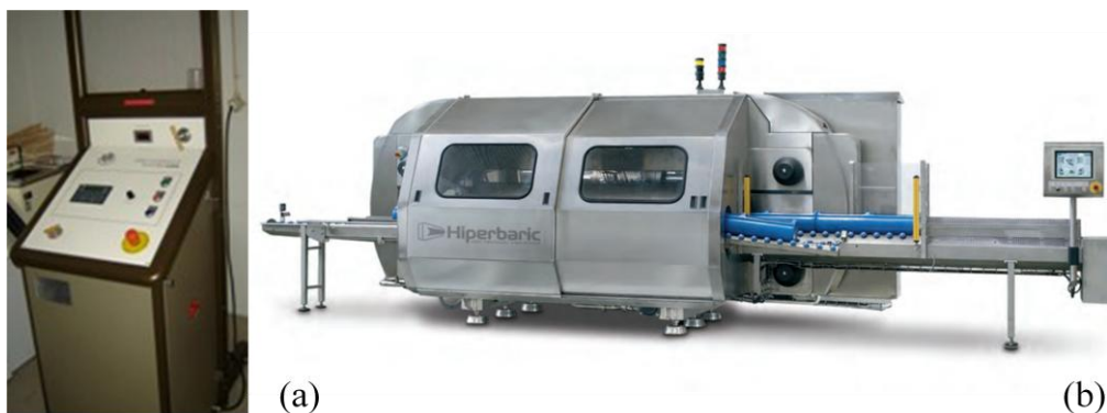
Figure 8. Hydrostatic presses used from hyperbaric experiments: (a) laboratorial scale and (b) industrial equipment.
