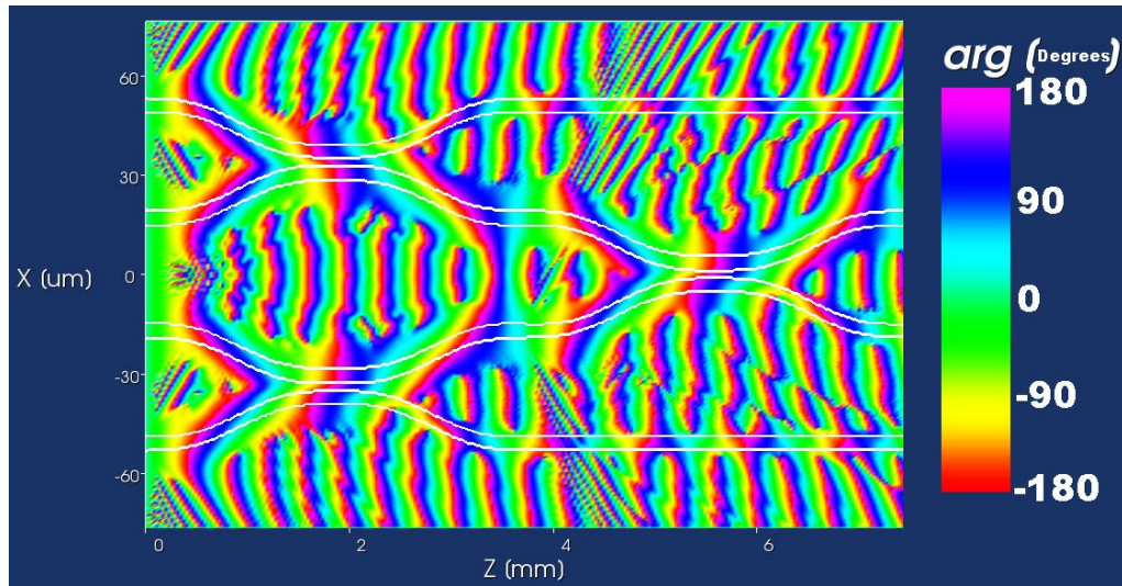
Figure 62: Phase propagation along the optical Haar transform schematic for Experiment 1 [22].
