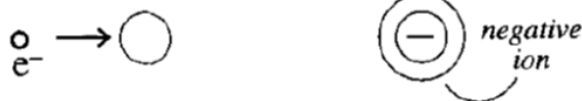
Figure 1.4 – Scheme of electron attachment, leading to the creation of a negative ion [17].
