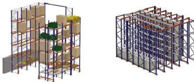
Figura 4. Rack Convencional e Rack Drive-in e Drive-through (fonte: www.hollyequipment.com ).
