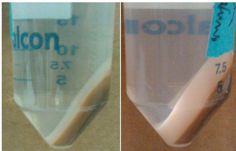
Figure 14 - Pellet of the mixed liquor sample of the growth reactor (left) and from the accumulation reactor (right) after centrifugation at 10,000 rpm for ten minutes.
