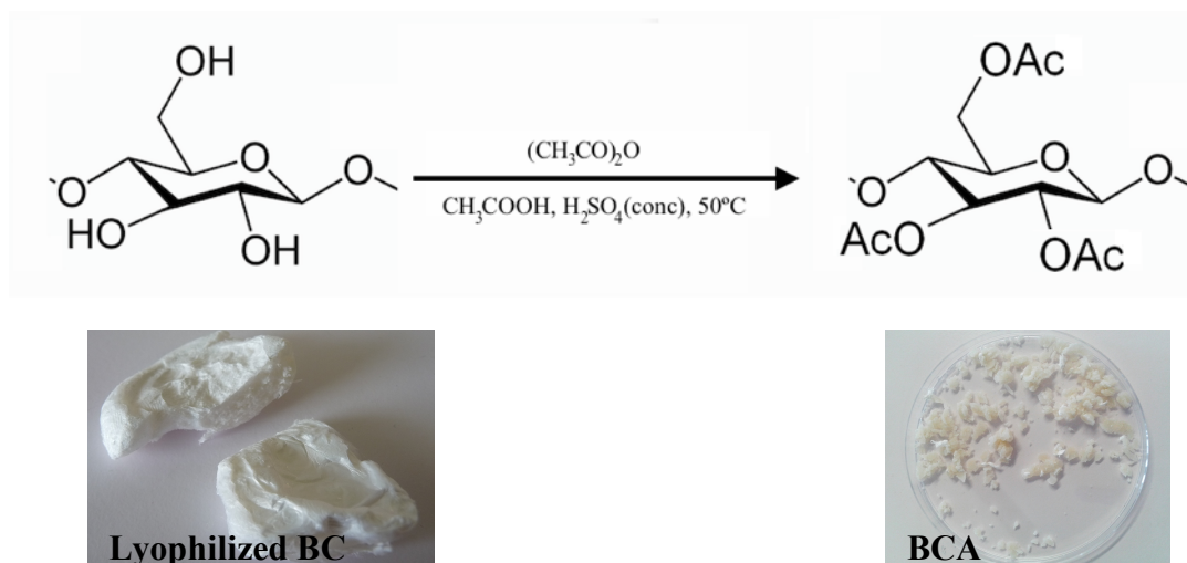
Figure 10. Schematic representation of BC acetylation and visual aspect of BC before and after modification.
