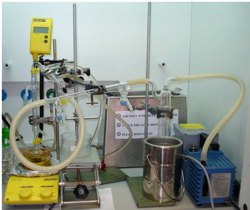
Figure 2.3- Experimental setup used for the D-xylose/[Emim]HSO 4 reaction system under reduced pressure (Chapter 8).
