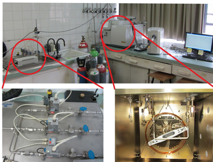
Figure 6.16 – Schematic representation of the instrumentation used for the separation tests: ( top ) overview of the equipment composed of flux gas controllers, a gas chromatograph and a mass spectrometer; ( bottom left ) flux gas controllers for different gases of interest; and ( bottom right ) view of the home-made chromatographic column packed with 29 inside of the thermostated GC oven.
