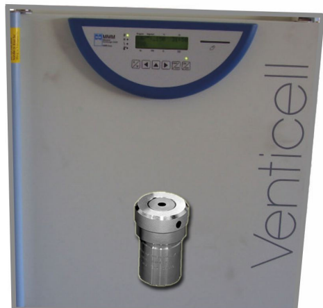
Figure 1.15 – Representation of the instrumentation used in hydro(solvo)thermal synthesis: oven and autoclave (inset).
