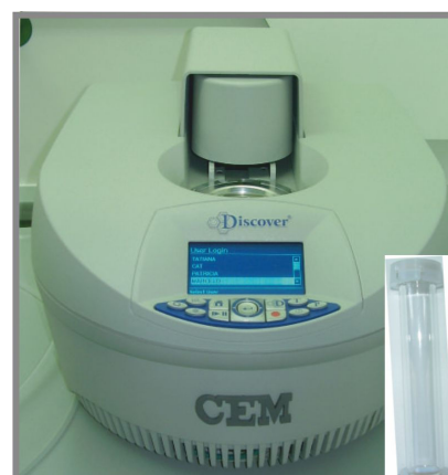
Figure 1.16 – Representation of the apparatus used in microwave-assisted synthesis. Inset is a common reactor for this equipment.
