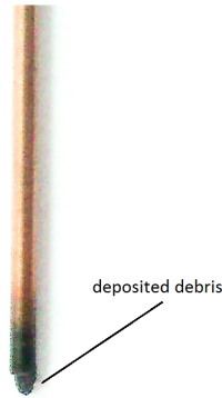
Figure 59 – Bottom surface of electrode used on first preliminary experiment
