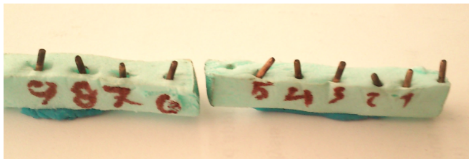
Figure 48 – Tips of the electrode tool used on the final experiment
