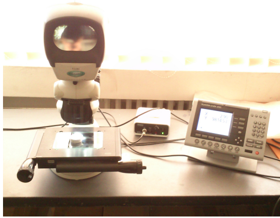
Figure 49 – Microscope Kestrel model and an microprocessor Quadra Check 200
